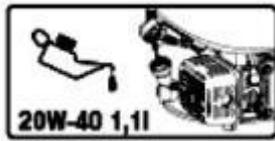
**check the oil tank before using, oil tank capacity refer to the engine manual.**
