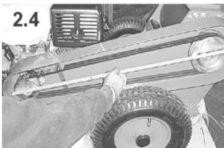
**Make sure that the belt is tightened , so that the belt pulley is aligned (Pic 2.4).**
