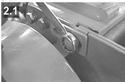
**Unscrew the locking screw of the engine (Pic 2.2)**
